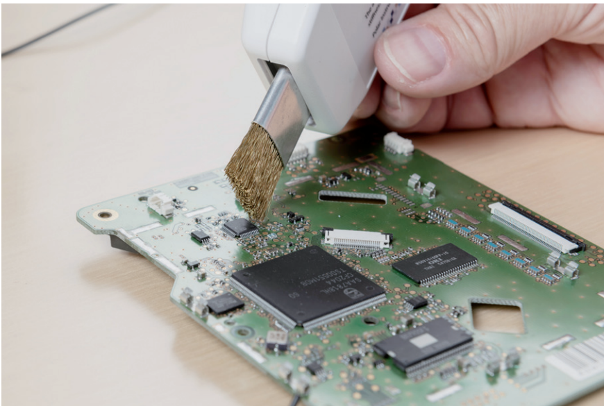
Use the edge of the brush to home in on the connection
