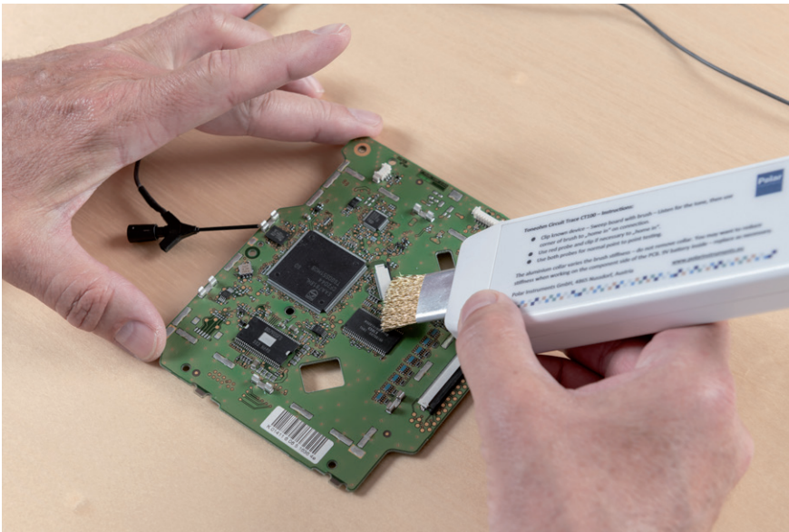
Probing the electronic circuit board assembly with the broad-side of the conductive brush
