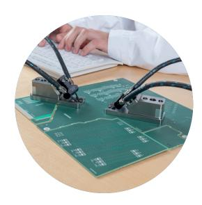
The Delta-L 4.0 De-Embedding Technique eliminates the effect of the probes, extracting the signal loss of the traces
