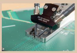
A pair of precision Delta-L 4.0 probes ensures optimum signal launch
