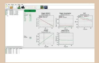
ATLAS VNA displays additional parameters such as Eigen Uncertainty, S21 of the short and long line, Phase and Er
