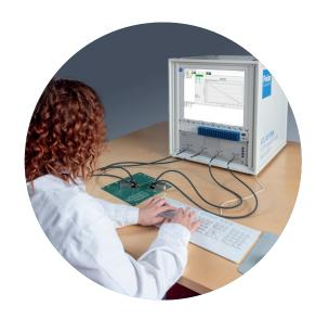
ATLAS VNA is a turnkey rackmount system and comprises all required probes and cables.
