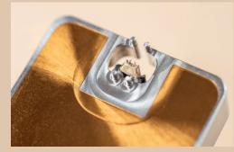
Delta-L 4.0 Probe Footprint with guidance pins
