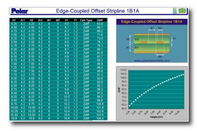
By extending the Sensitivity Analysis featured in the Si8000m or Si9000e, the Si Excel interface allows you to graph any parameter using the pre-prepared Microsoft Excel workbooks or to build your own workbooks to model your process.
